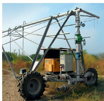
The linear irrigation machine allows to carry out effective irrigation of rectangular fields in the automatic mode.
