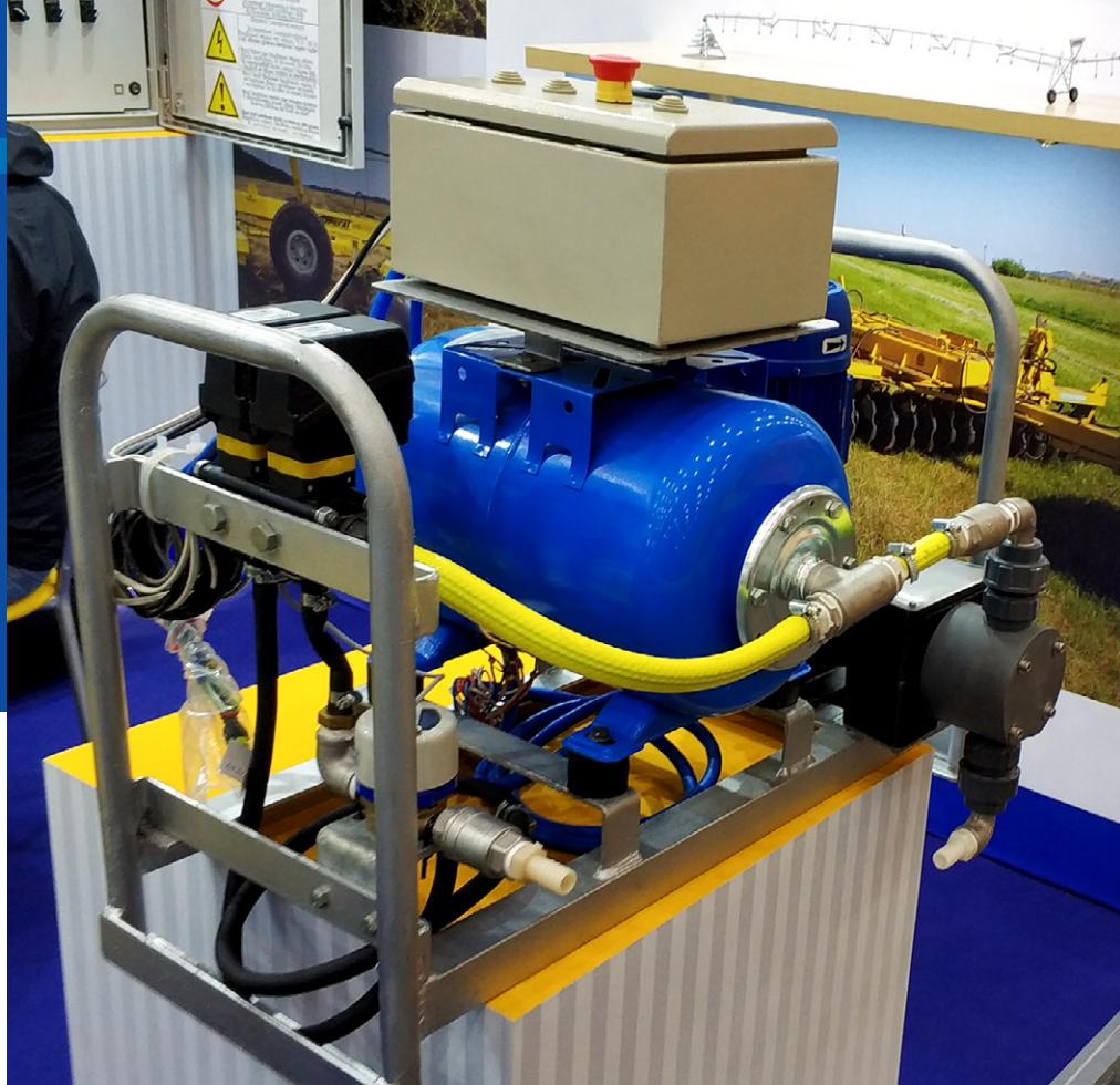
The fertilizing aggregate unit is based on the Seko Spring PS2 (Italy) plunger-type dosing pump.
