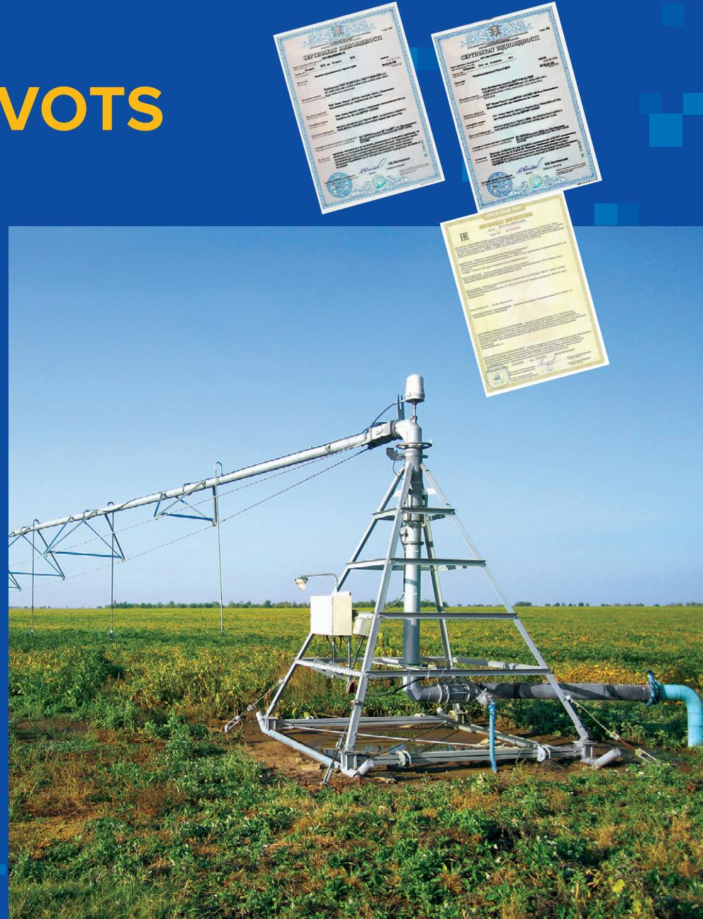
The DMF Fregat irrigation machines of pivot modification are able to execute the automated irrigation via the dynamic revolving movement around a stationary support.
