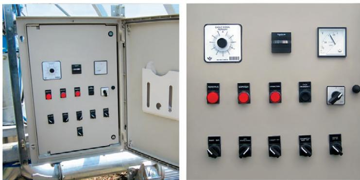
At the current moment, the control cabinets are available in two versions: the relay and controller-relay ones for center pivot, linear and hippodrome machines. Later, the third version will be mastered – the controller one, akin to a controller-relay system with a touchscreen, but without manual control with switches, buttons and light bulbs.
